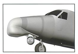
With integral fuel tanks and the two largest sensors with associated LRUs in the nose section of the aircraft, the cabin is free for mission operating crew, observers and for ancillary payload, thus maintaining full multi-role versatility of the aircraft.
